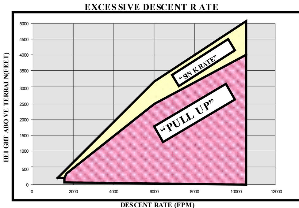
**8.0 CLASS B EQUIPMENT TEST REQUIREMENTS FOR NEGATIVE CLIMB RATE OR ALTITUDE LOSS AFTER TAKEOFF.** Use the existing performance envelopes specified in RTCA/DO-161A based upon a “Height above Runway ” using barometric altitude (or equivalent) and runway elevation in lieu of radio altimeter inputs.
